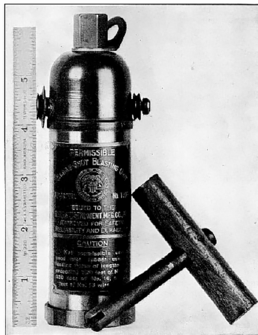
FIGURE 12.—Assembly view of Davis No. 66 magneto-type unit, approval No. 1203
