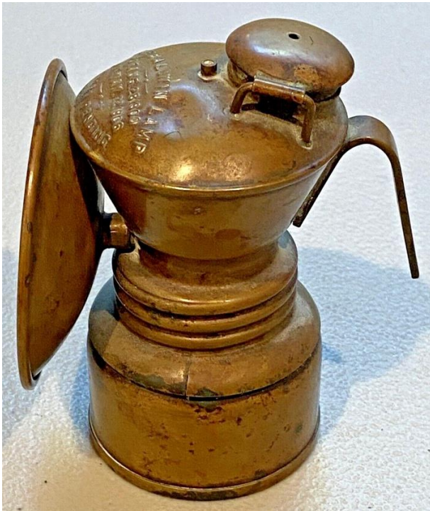
Rolled-edge brass reflector with Michigan spade (unknown collection). The author has seen three lamps identical to this, and all have a split in the push-on tube which is made of very thin material.
