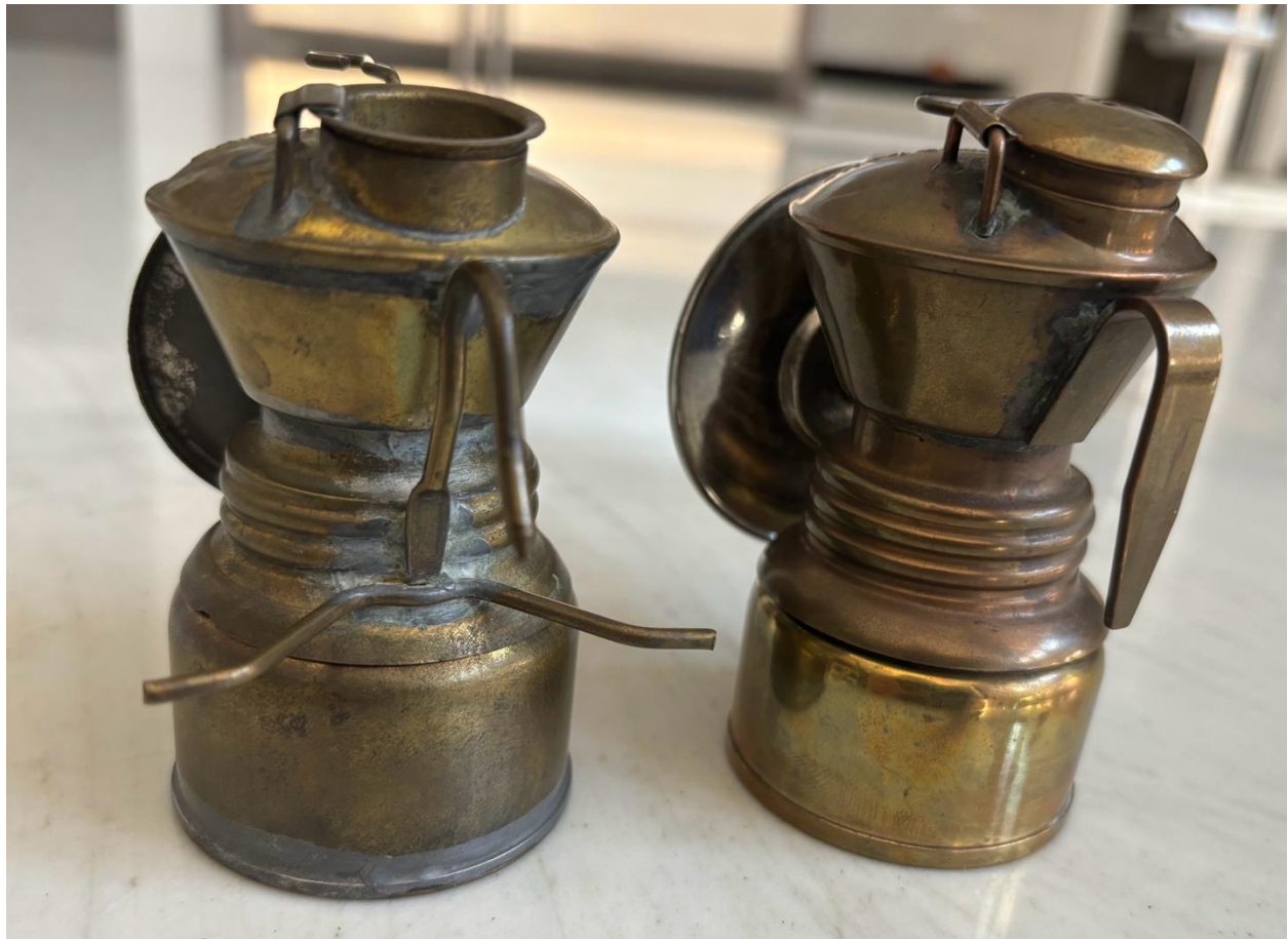
Baldwin mounts showing the classic hook and brace mount compared to the "Michigan Spade."
