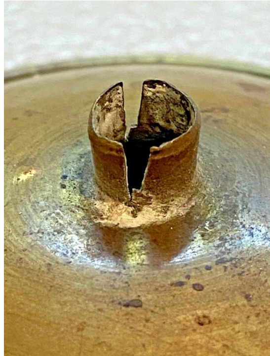
Rolled-edge brass reflector with Michigan spade (unknown collection). The author has seen three lamps identical to this, and all have a split in the push-on tube which is made of very thin material.
