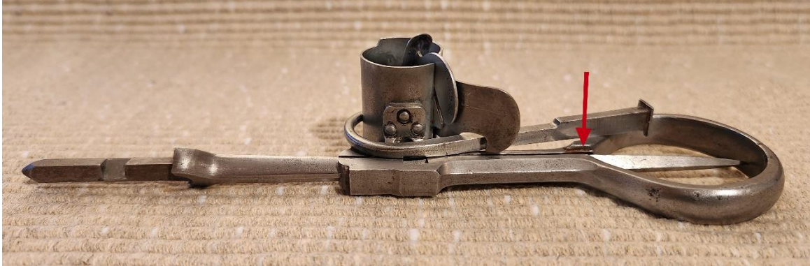
Type B: Reassembled for pocket-carrying but still loose and not locked. Note raised locking ridge on the handle (arrow)
