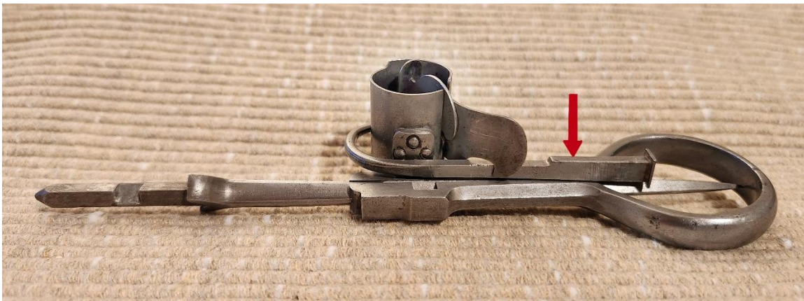
Type B: The stem of the hook is pressed down over the locking ridge (arrow), tightening it against the thimble lever and also locking the snuffer plate tightly inside the thimble.
