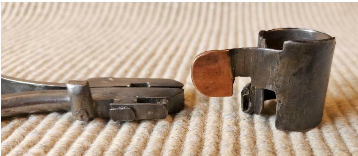
The Type D handle showing Roger's repair of the mounting flange and the added locking post. The original Werntz-made thimble with copper thumb lever has been fitted with a slot for the mounting flange.
