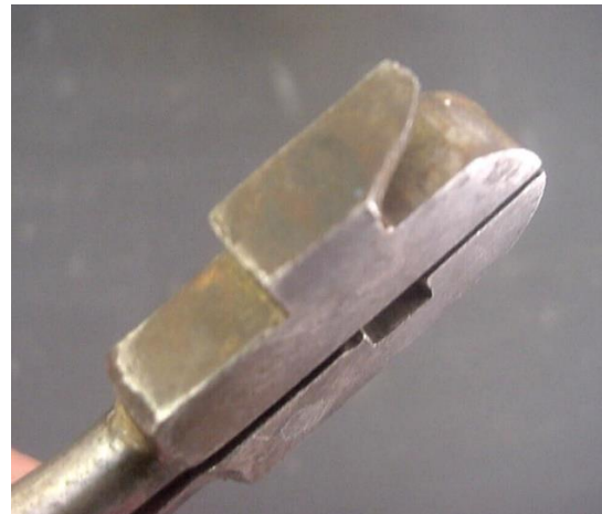
Handle neck area of the Type D handle showing broken flange.
