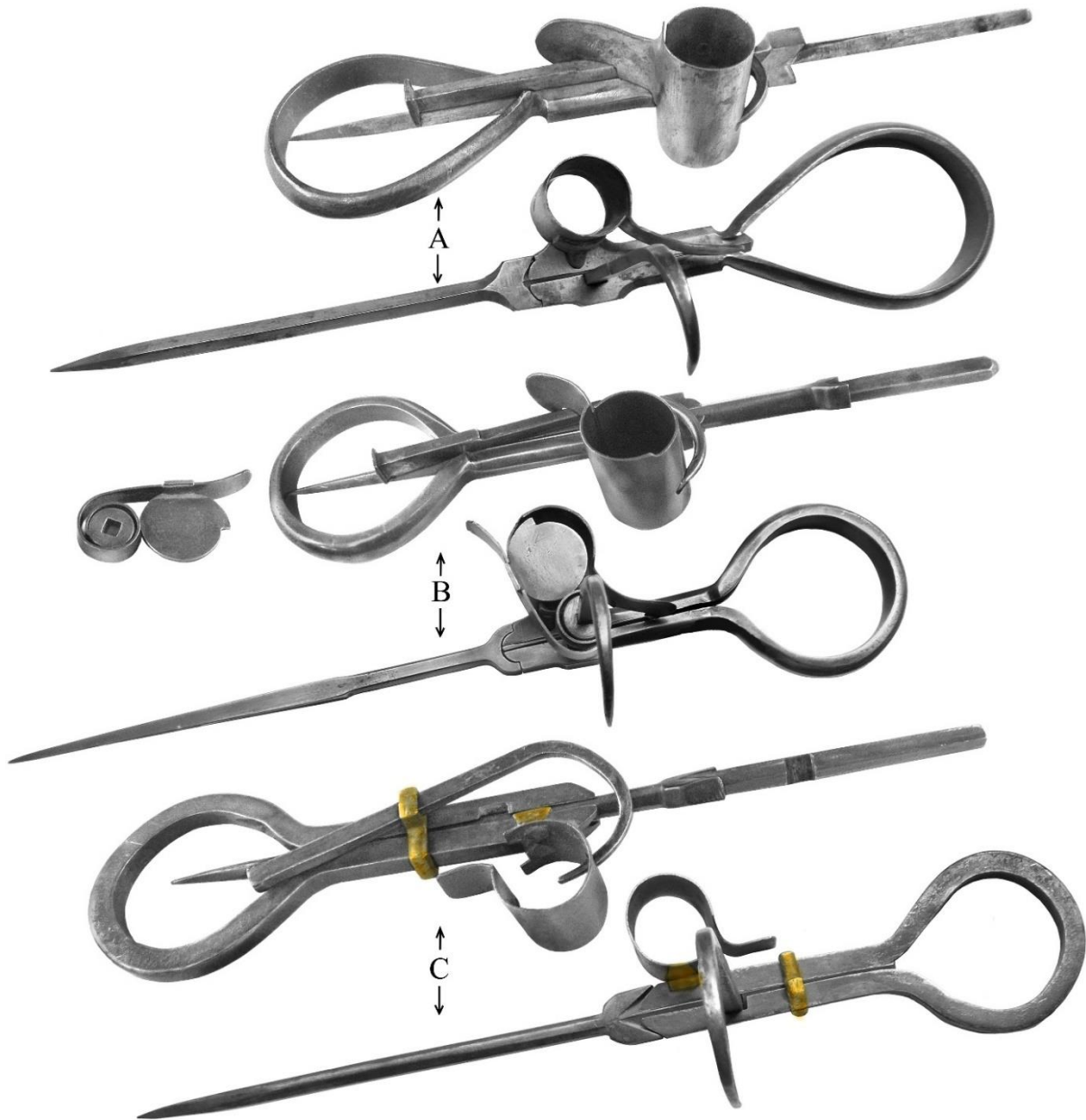
The three main types of Gabriel Werntz candlesticks, shown in the stowed and working configurations. Al Winter collection.
