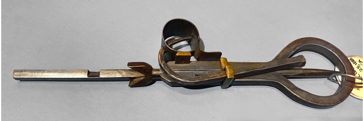
The Type C Werntz in the stowed configuration (note dovetailed thimble mount).
