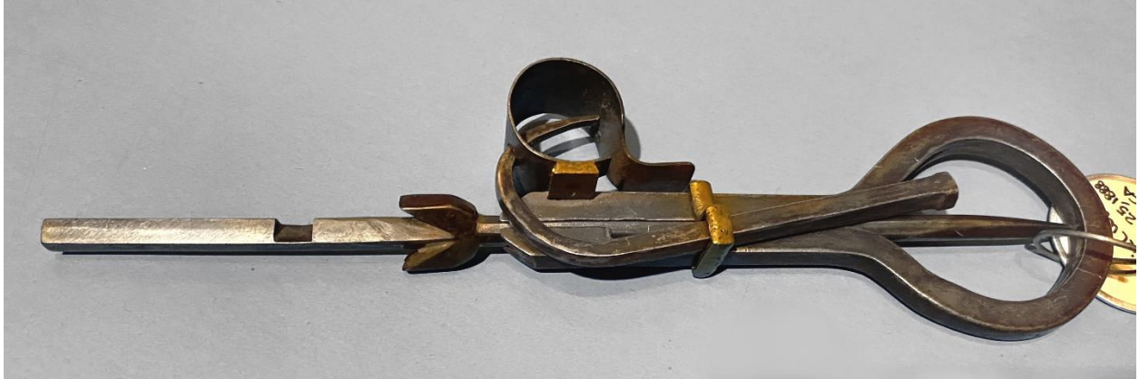
The Type C-1 Werntz in the stowed configuration (note dovetailed thimble mount).
