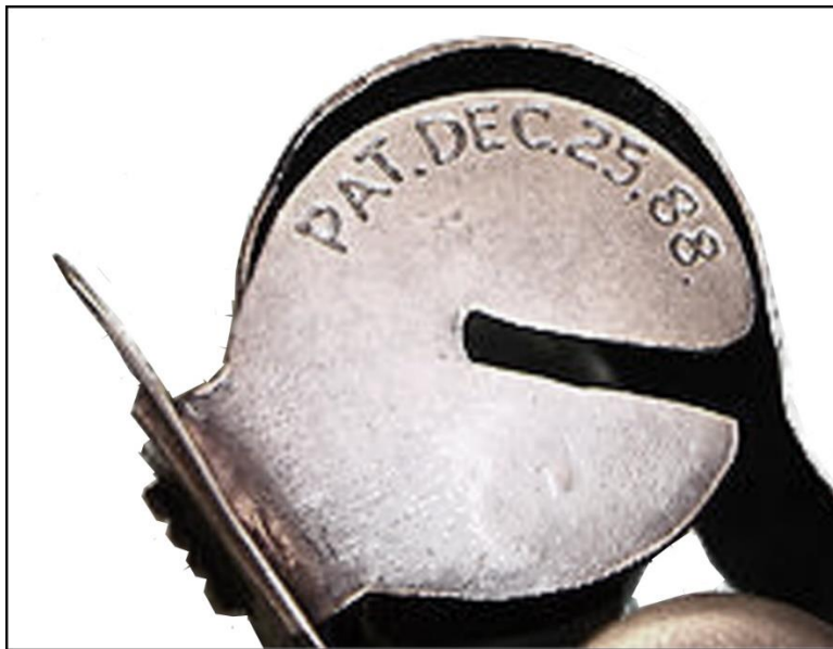
This is the lid of the Worthpoint reproduction snuffer, said to be marked "#3" on the bottom side. The cutting of the slot is rougher than with original snuffers, and the engraved (rather than gangstamped) lettering is thicker and less precise.
