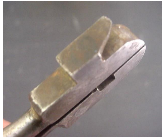
Handle neck area of the Type C-2 handle showing broken flange.
