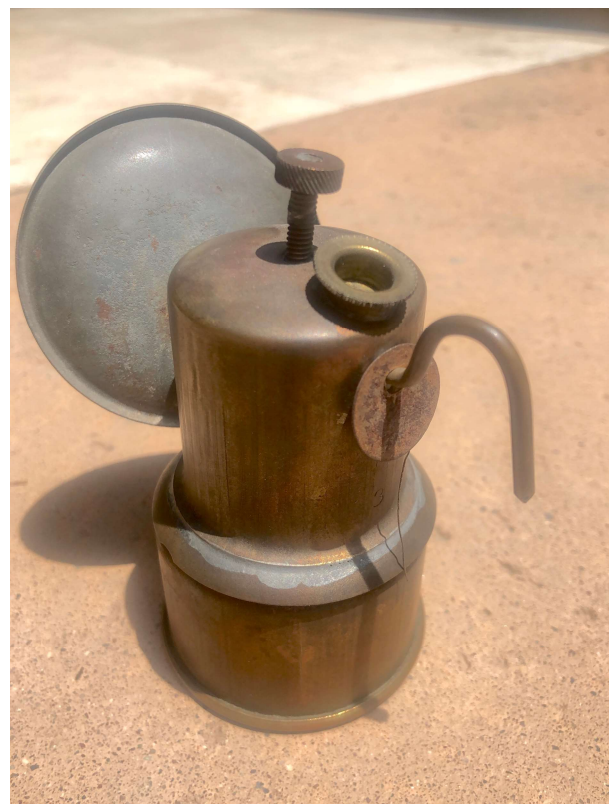
Left: Early Baldwin hand lamp with disc tip cleaner hanging from wire hook on water tank. Right Victor cap lamp with disc tip cleaner hanging from cap hook. Author's collection.
