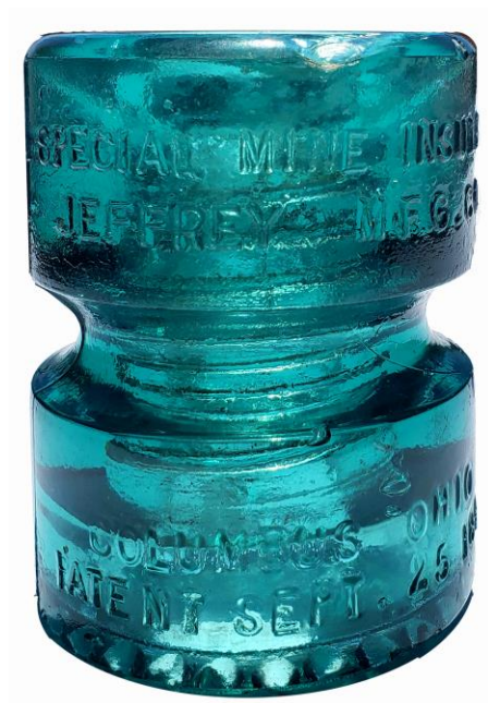
“SPECIAL MINE INSULATOR” “JEFFREY MFG. CO.” (embossing right-side-up) Hemingray-made CD 185 (author’s collection)
