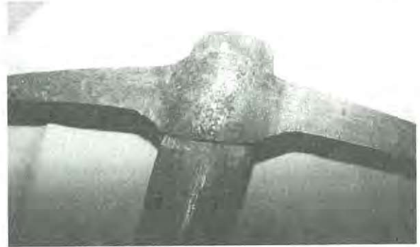
Figure 4. Typical features of a pickhead made with the Collins Process. Note the crescent-shaped flange embracing the handle under which are slits at the apexes of the socket. On the left tine is the "Collins & Co./Hartford" gangstamp. (Author)
