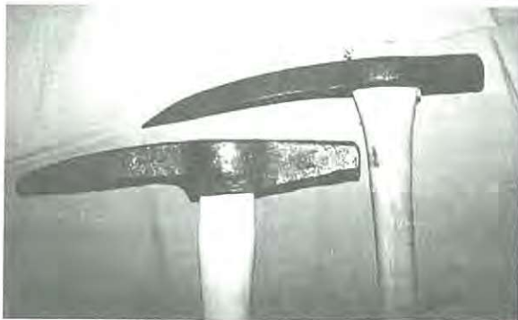
Figure 3. Two types of hand-forged poll picks. The top pick with its flat profile is most characteristic of hand-forged pickheads; the other pick features an odd profile uncharacteristic of machine manufacturing. In addition, it has slits at the apexes of the handle socket where it was spread. (Author).
