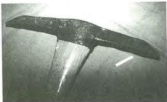
Figure 6. This drift pick was manufactured with the Bealor process. Note the ragged edge of the handle flange and crude forge-weld where its two halves were joined. The arrow points to the spot where the hardened steel tip was forge-welded onto the end of the tine. It is deformed due to blacksmith-welding and resharping. (Author)
