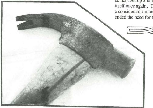
The head of a Homestake claw hammer that was made by the Homestake Mine in its foundry. (Chuck Tesch collection)
