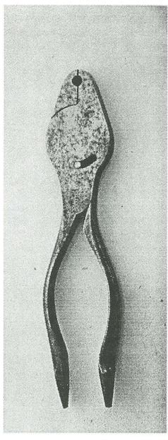
I picked up all three of these crimpers from Nelson Ressler some time ago. They are all different, but appear possibly to be made by the same company. None are stamped. You can see a small pin in a slot in each plier that limits the jaw opening. The crimper on the far left has a tapered hole. The other two just go straight in. If anyone can help identify the manufacturer I would be most grateful.
