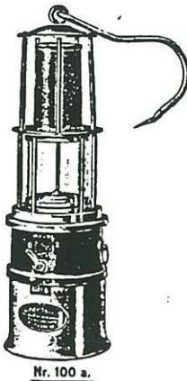
Carbide safety lamps. Lamp on left is fitted with an additional water regulation.
