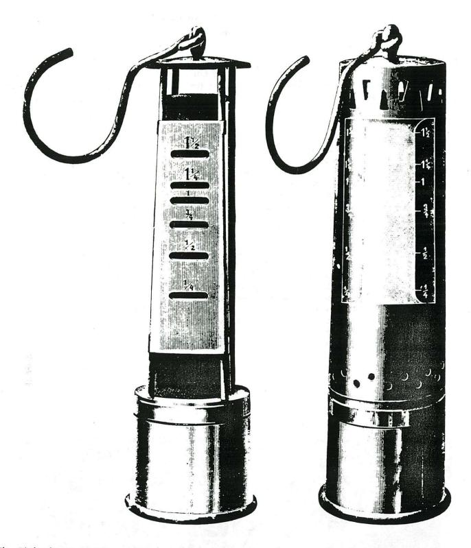
The Pieler lamp was an extremely poor choice for any other use other than mine gas testing. In the presence of gas, the lamp would heat up quickly and when the concentration was high, the flame would fill the lamp. Intended to detect gases when the concentration was too small for measurement with a standard Wolf type safety lamp, the Pieler would almost inevitably cause an explosion if brought into the presence of a substantial body of gas.
