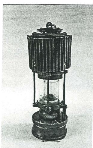
Class of lamp: Safety Lamp for Oil burning Type HCP
