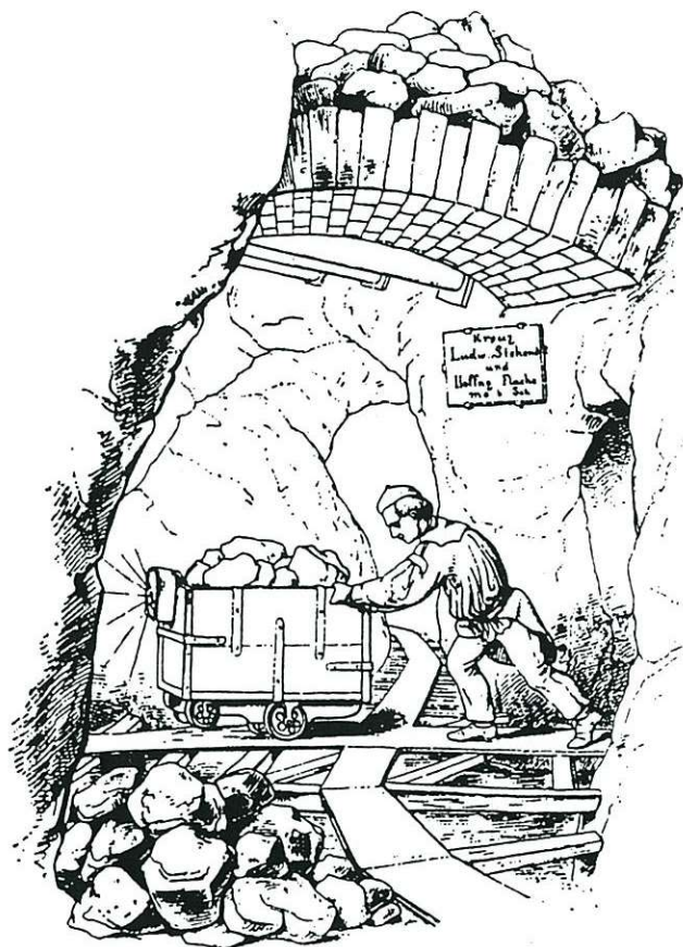
Figure 2. A trammer with his Blende hung on the front of the ore car (illustration from Eduard Heuchler's Des Bergmanns Lebenslauf , 1867).
