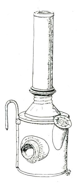
Perhaps one of the more interesting miner's oil lamps patented was that of David D. Williams. The most unique feature of this lamp is the screw-on wick cover that is cleverly designed to double as a lamp handle. The patent text describes these features and mentions its leak resistance while carrying the lamp in a pocket, but makes no mention of surveying. An advertisement which does list such a lamp as a surveyor's lamp has been reported, but has not been seen by the author.
