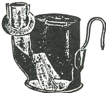
Sectional View, Showing Heater
