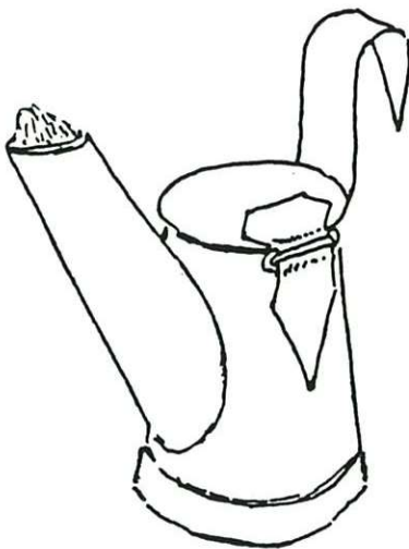
DL lamp, 55 mm high (measured from lid to bottom). Tin with brass reinforcing ring and flat steel hook.
