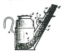
This lamp's most unique feature is a mechanical wick raiser that consists of a brass knurled knob connected by a shaft to two brass five pointed "wick engaging wheels" housed in a semi-circular housing mounted on the top of the wick tube. This housing allows the pointed wheels to sit approximately half way into the diameter of the wick tube to engage the wick. Guess what? It really works!
