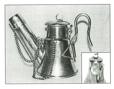
The spout is 3" in length and ¾" in diameter at its end. A rarely seen accessory on the spout is the cap which is connected by a chain to the piece between the spout and font. Crossed hammers on the end cap suggest a European influence. Like
