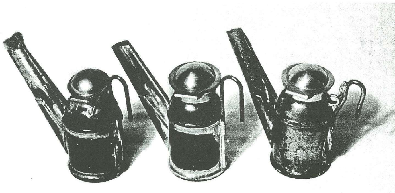
Left: previously described lamp without the patent . Center: new style lamp without the patent. Right: new style lamp with patent. All three are Trethaways.
