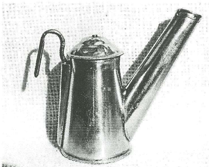
(above) Unmarked oil wick made of German silver w/ brass bottom, hook, and vent tube in the cap.
