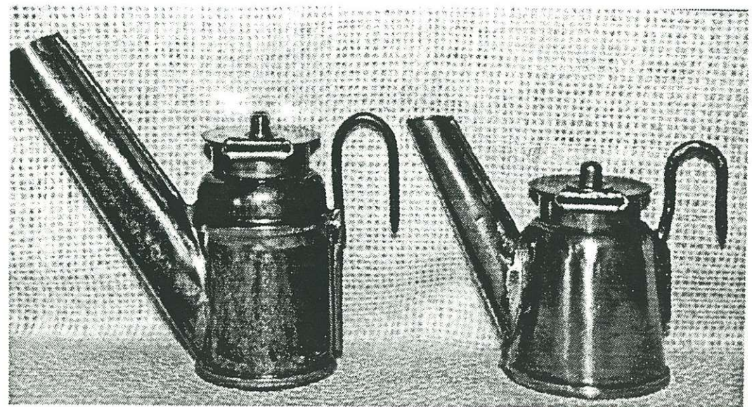
Left: tin face lamp with brass collar and cap and stamping B, G, and I.
