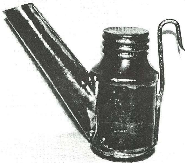
This unusual Zais lamp has straight sides and a sharply angled shoulder with a screw-on lid.
