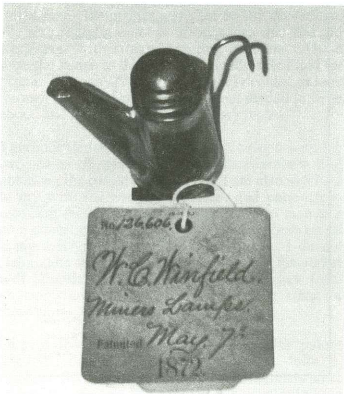
The improved Winfield lamp of 1872. Lamps were mass-produced under this patent.
