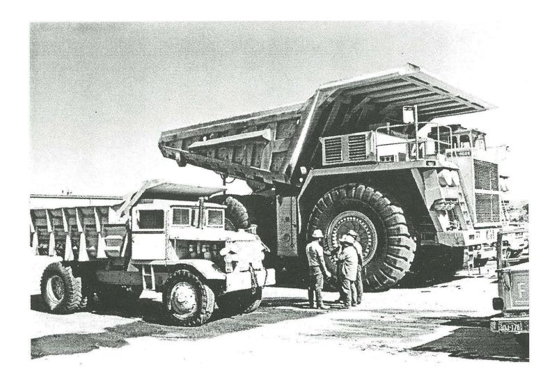
here is more than just a little difference in these two trucks, one is a 1940 Euclid, 30-ton ore truck. The other is a 1991 Dresser Haulpak 685E, 190-ton ore truck. It's pretty easy to tell one from the other. Fiftyone years and a lot of technology is the difference. The 1940 Euclid started its mine life at the Castle Dome mine 12 miles west of Globe, Arizona. The Castle Dome Mine was a copper mine funded by the "Defense Plant Cor-
