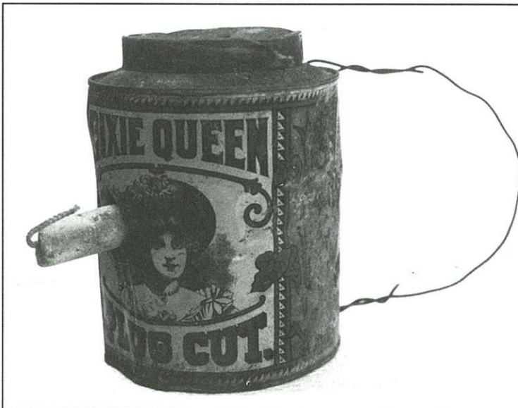
Bug lamp from the Queen Esther mine. This one is not made from your usual Log Cabin syrup tin, but from a Dixie Queen Plug Cut tobacco tin.
