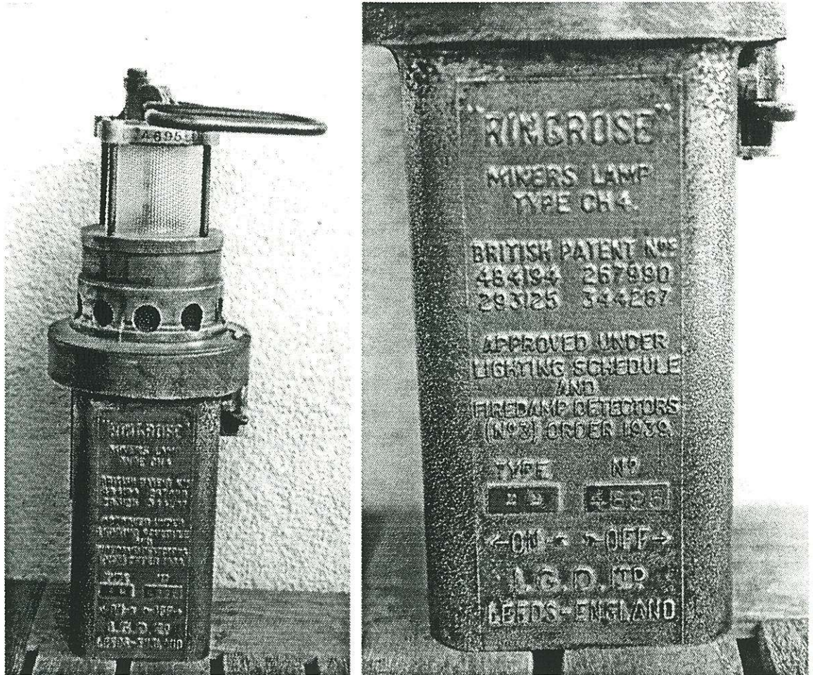
Right: Front and back views of the Ringrose firedamp alarm Type: CH4/DB.
