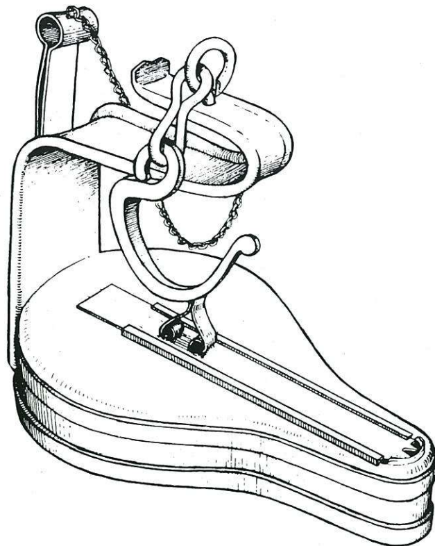
Figure 50. Steiermark Frog. This example, made by Franz Grebenz, Trefail, in Steiermark, is rather similar to the previous illustration. The unusual hook and the bands about the front serve to distinguish it. It may have carried a reverse-facing shield originally, which is now missing, though many similar examples have no shield. (Drawn from another drawing, not a photograph, so details are less reliable.) Late 1800's. (Owner unknown)
