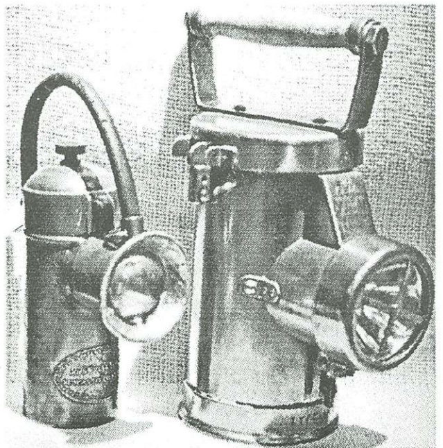
Left: Copper Joel-Fors Patent lamp made by John Mills & Sons. Right: CEAG inspection lamp, Type BE, all brass.
