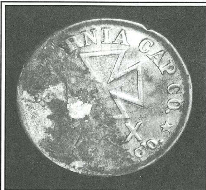
One side of a rusted lid of a California Cap Company tin cleaned by the electrolytic process described, other side untreated.
