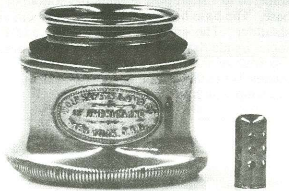
1921 cap lamp bottom showing company name tag, water spreader, and unique threads
