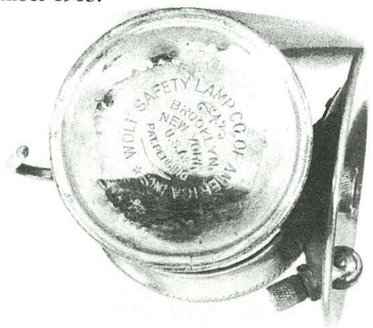
Soldered bottom seam, 1923 Wolf cap lamp
