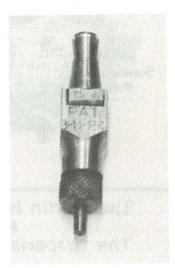
The Shanko Device fits in the lamp's burner tube and the tip is fit into the cleaner. The cleaning action is as follows. The knurled nut and plunger is spring-loaded and pulled out as the device is swung into horizontal position. When released, the illustrated cone fits into the depression at the center of the burner tip. Inside the cone is a fine wire which is pushed into the burner hole when the plunger is depressed.
