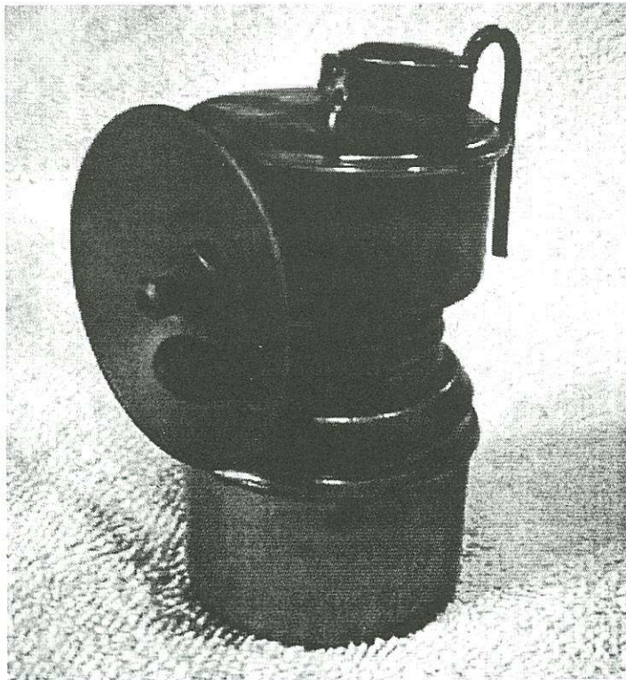
(left) Stein Dropper lamp, an imitation of the Guy's Dropper is shown here with 2-inch steel reflector. (above) The rear view shows the reflector to be rolled flat back against itself.
