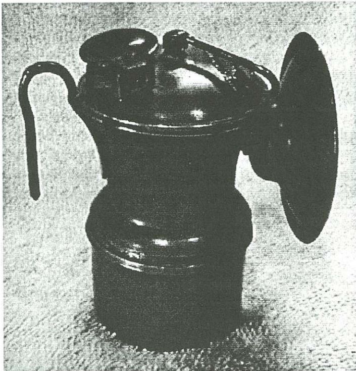
Early Springfield Lamp with sharp-edged reflector. This reflector belongs on water tanks with a sharp-edged skirt.
