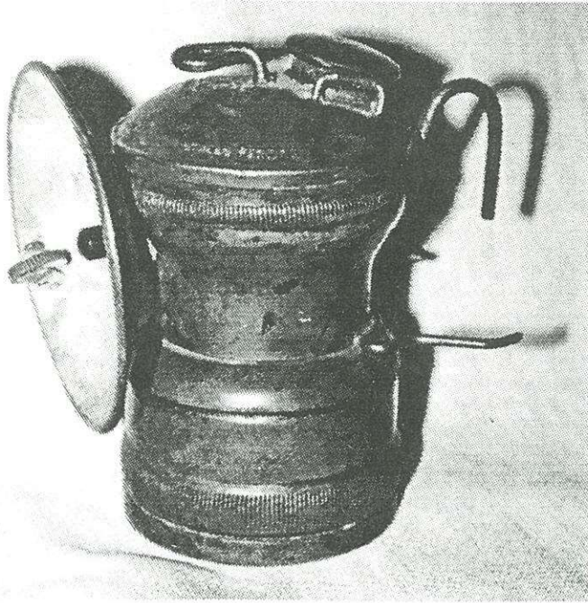
Most basic model with heavy bent raking wire, no tank notches. Brass.
