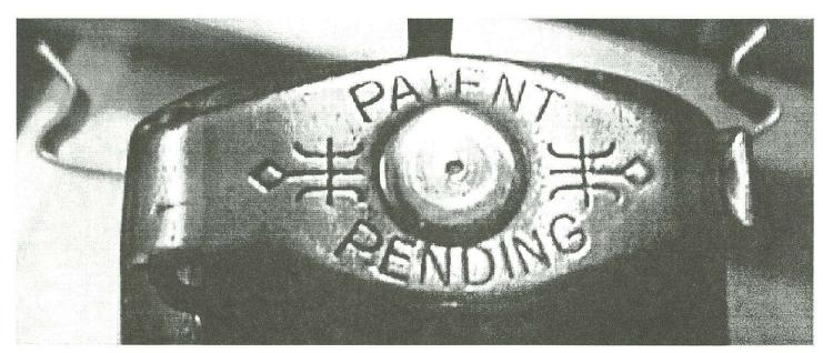
Justrite cap lamps with a special waterdoor were sold during the 1919-1920 period. They featured a fancy stamping and rubber gasket to make a tight seal with the lamp hole. It one of the most difficult of all Justrites to find today.
