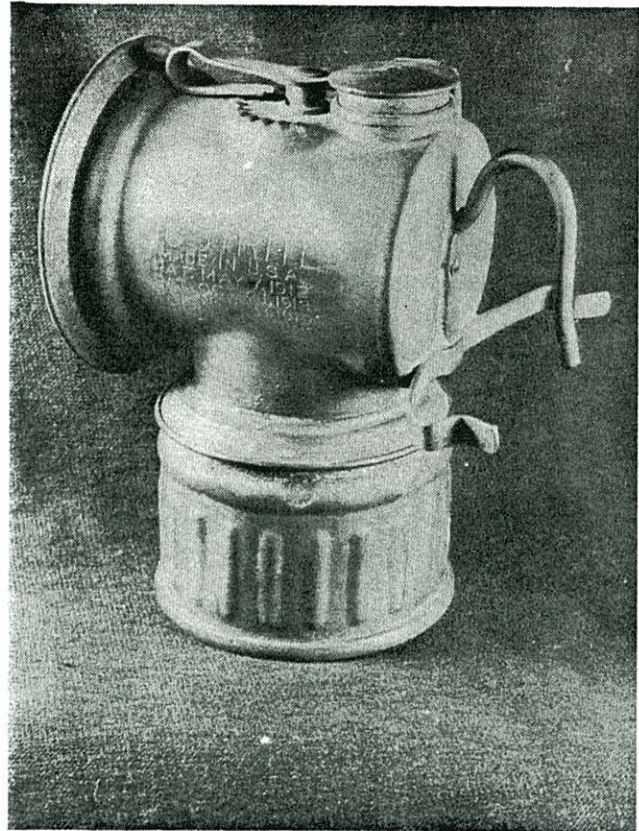
The "Polygon Pat. App. For" lamp (ca. 1922) showing change to round water door and thinner rear brace.
