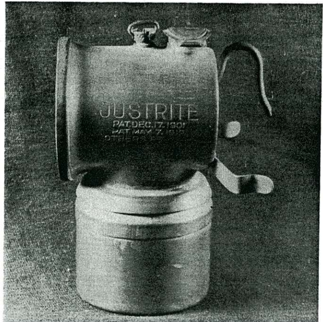
The "Miners' Pit Lamp". The primitive raking wire is still present, but the knurled wheel water cut off is now deeply notched. The stamped name has been shortened to simply "JUSTRITE". (Dave Thorpe collection)
