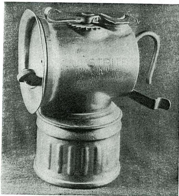
One of the first cap lamps of the Frisbie era (ca. 1920) shows ribbed base, "MADE IN U.S.A." stamping, and increase in number of lever bumps from 12 to 16.
