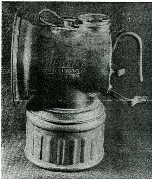
Above: lamp made in late 1920's showing changes to raised lettering with only one patent date. Also note round ringed water-door with thumb tab, and shorter water-lever.
