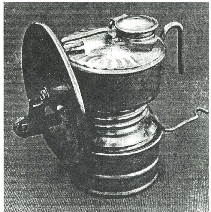
Late "One-Date" lamp with clamp-on striker (Dave Thorpe collection.)
