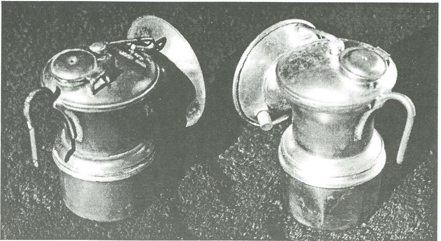
Only two reflectors are acceptable for the Springfield Lamp. On the left, is the sharp edged version. On the right, the reflector has a crimped over edge.
