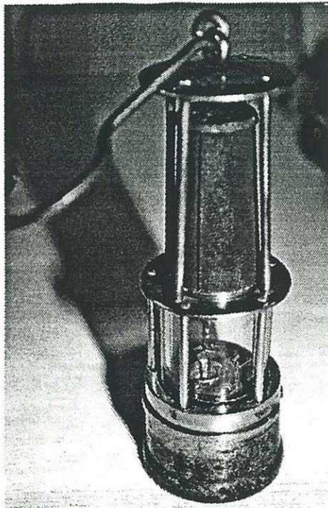
Early oil safety lamp with paper strip igniter.
