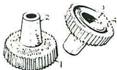
Enlarged reverse views of the "Bess" Burner. Length overall, \frac{3}{8} ". Greatest diameter \frac{3}{8} ". 1 is the tapered shank; 2, the milled edge; 3 and 4, water grooves provided to lead water around the gas flame.
