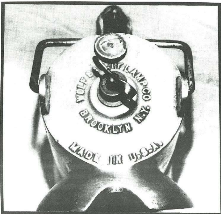
Figure 6. Top view of another Wolf cast aluminum 8-hour hand lamp showing the changes in the stamping. (Errol Christman collection)
