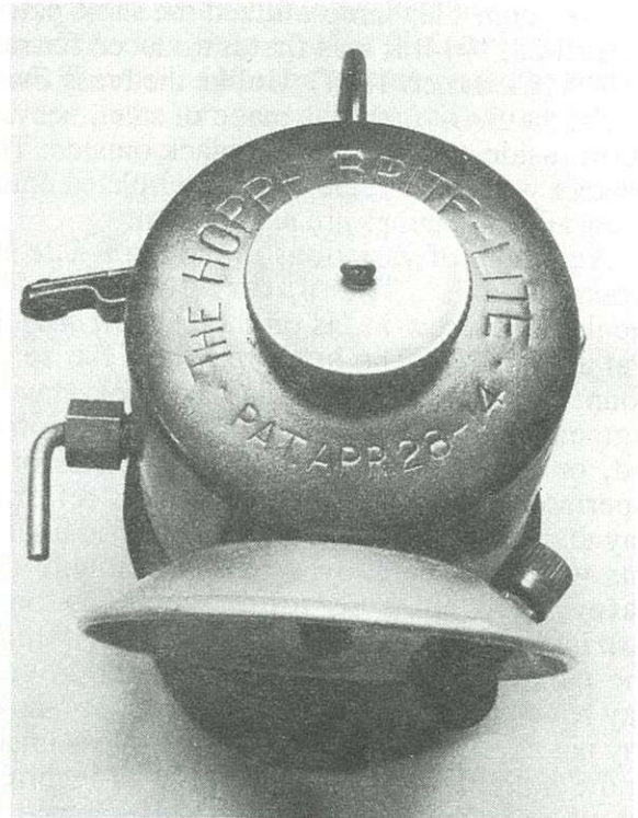
Figure 4. "The Hoppe Brite-Lite" with wire cap hook and flat brace. (Mike Puhl collection; photos courtesy of Dave Thorpe.)
