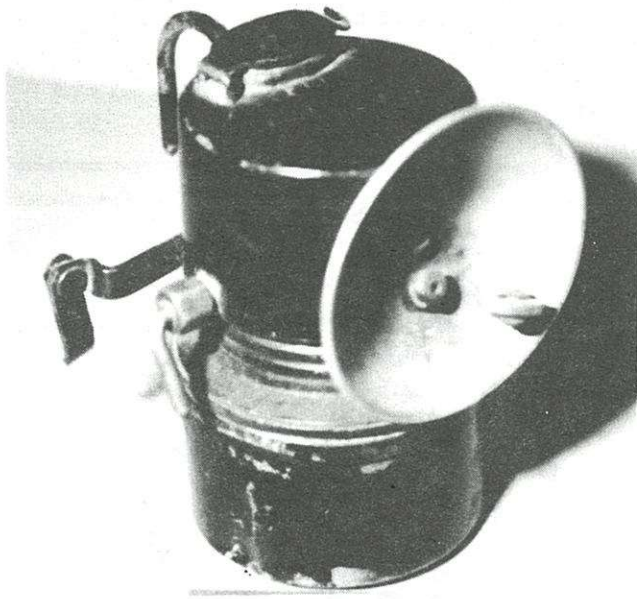
Figure 5. Harker Brothers "Brite-Lite" with oval water door, wire cap hook and hinged brace, and side-mounted water feed. (Dave Johnson collection)
