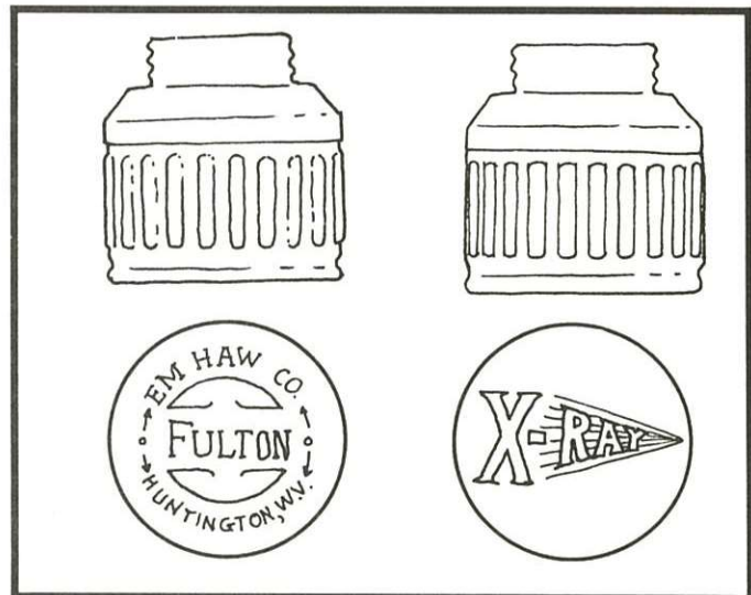
Bottom stamping of the Fulton cap lamp as compared to Justrite's X-RAY. (Illustrations by Wendell Wilson)
