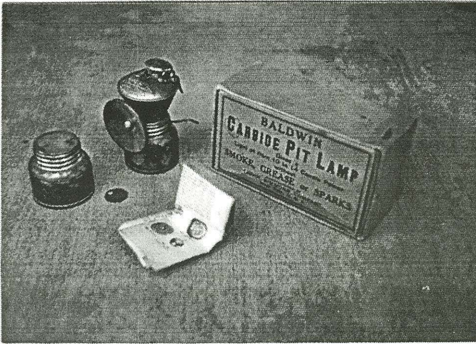
Baldwin lamp ca. 1911 with original box and shipping package. Note the burner tip cleaner on the metal disc. From the White brothers collection. Photo courtesy Dave White.
