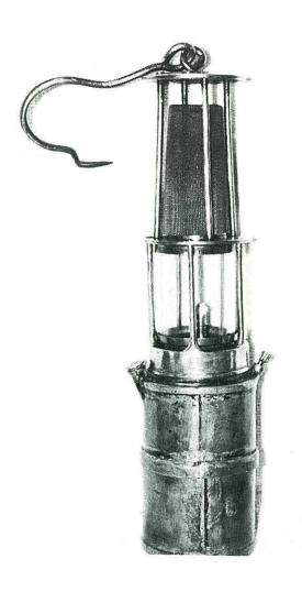
Carbide was naturally seized upon as a substitute for oil in safety lamps just as it was in cap lamps. However it never enjoyed the success in safety lamps that it did in cap lamps. At least three major European mine lamp manufacturers developed safe and efficient carbide safety lamps. Carbide safety lamps never enjoyed any level of acceptance in the United States. Unlike the oil fueled safety lamps, the carbide safety lamps produced 10 candlepower.
