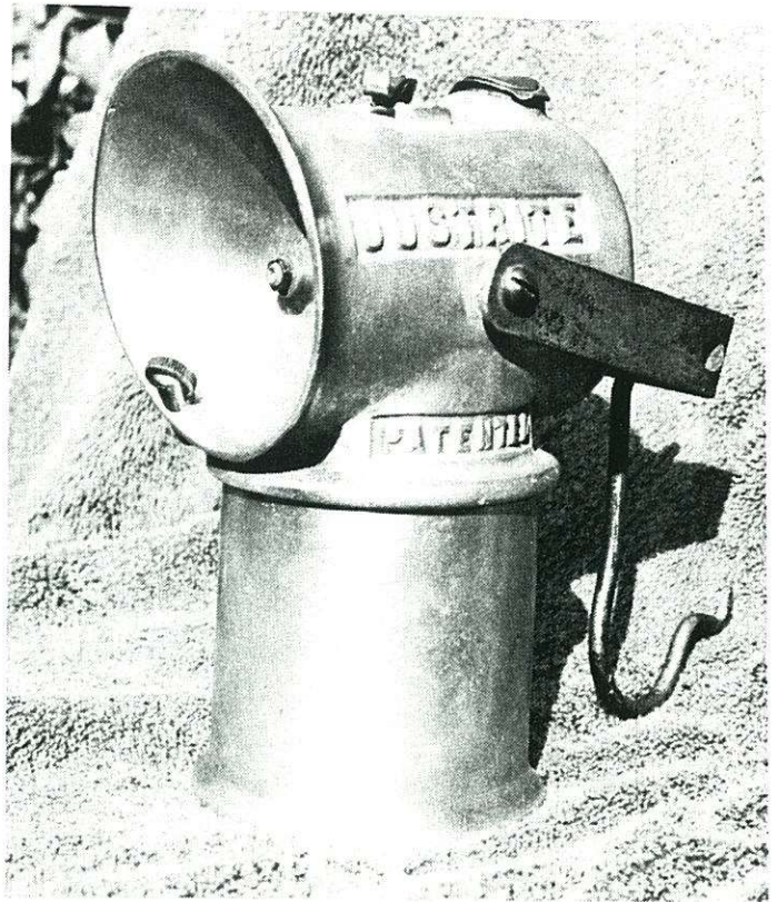
Fig. 1 Jumbo with central burner, oval door, "Patented" stamping and holes in bail for stick.
