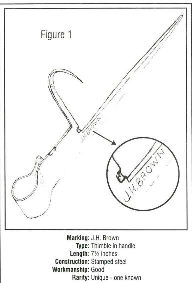
forging out of one piece of metal. Although the item is very rusty and pitted the edges, thicknesses, radii, etc. all seem to have been very concise and clean-suggesting this item was mass produced (as opposed to being a one-of-a-kind blacksmith model). The gang stamped name (assumed to be that of the Manufacturer) J.H.BROWN as well as the absence of excessive file markings, also seems to support the mass-produced theory. The metal used to construct the stick is very high
