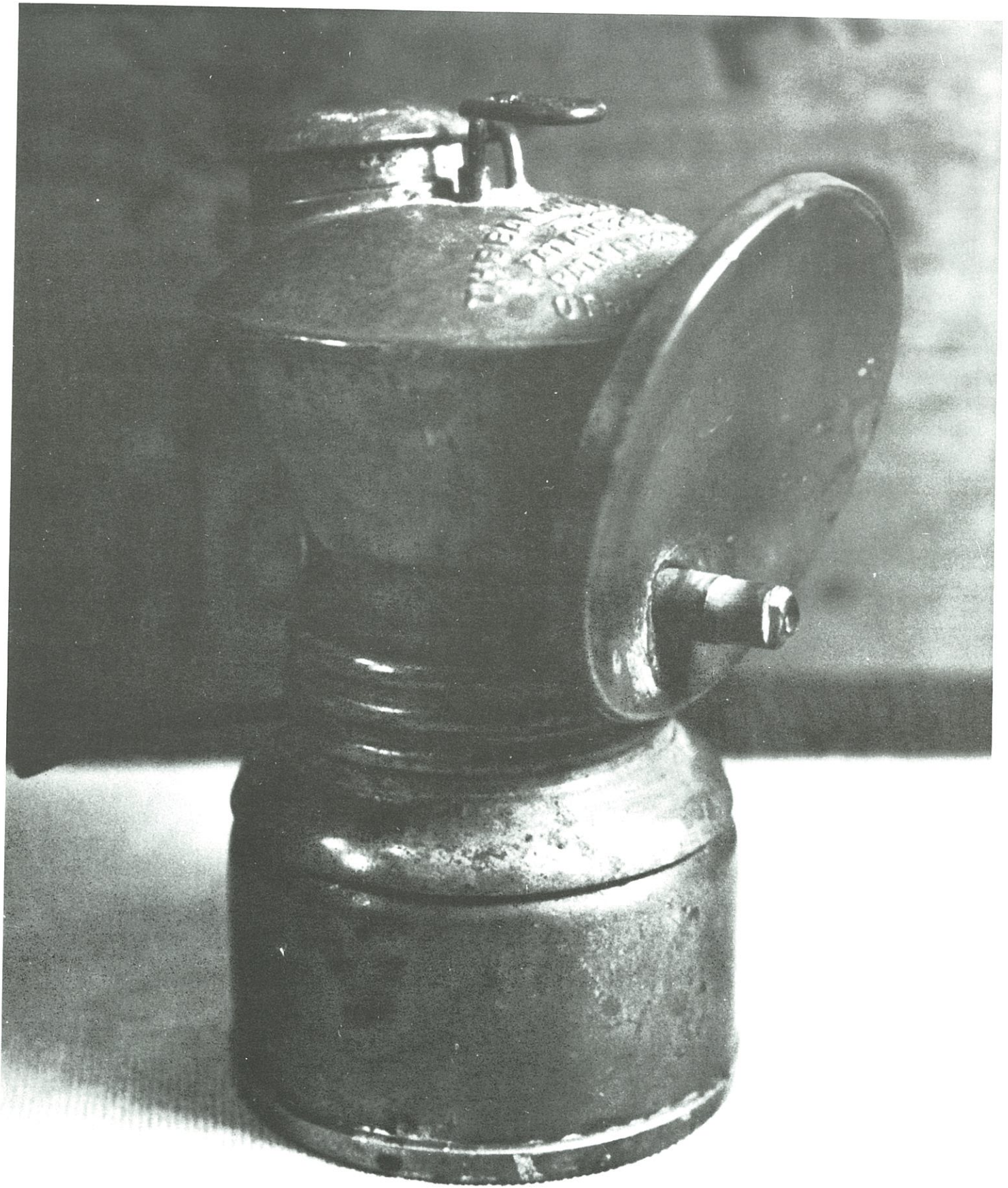
Baldwin lamp with tilted reflector and offset burner. (Dave Thorpe)
