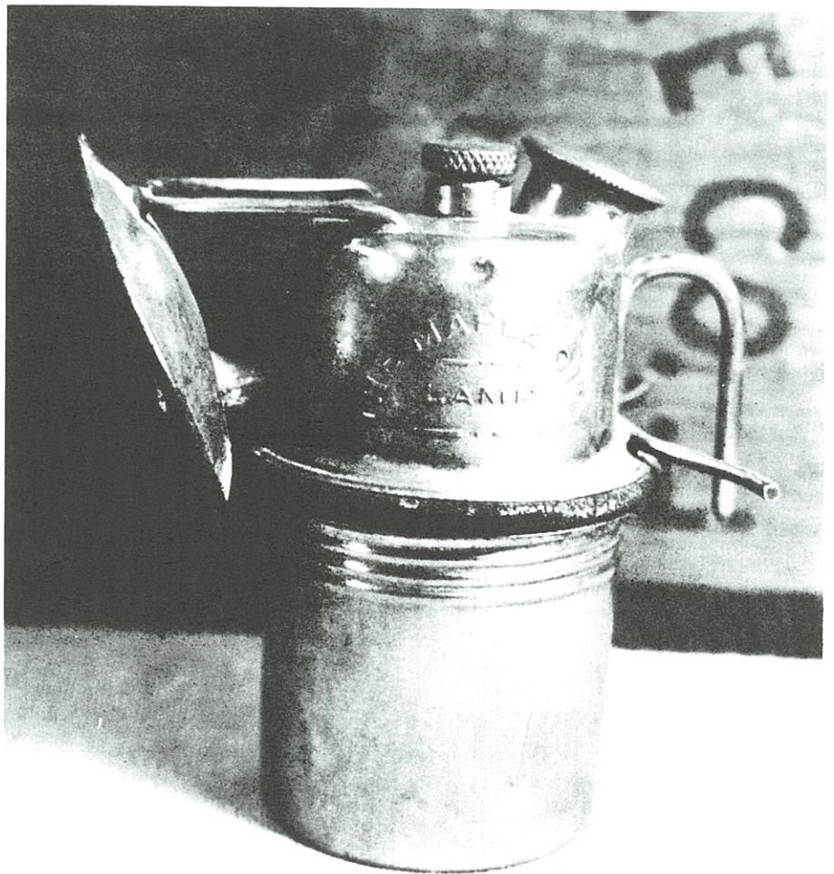
(above) Nickel plated and black painted Britelite lamps. Both have tilted reflectors and a low-mount burner. (Dave Johnson)
