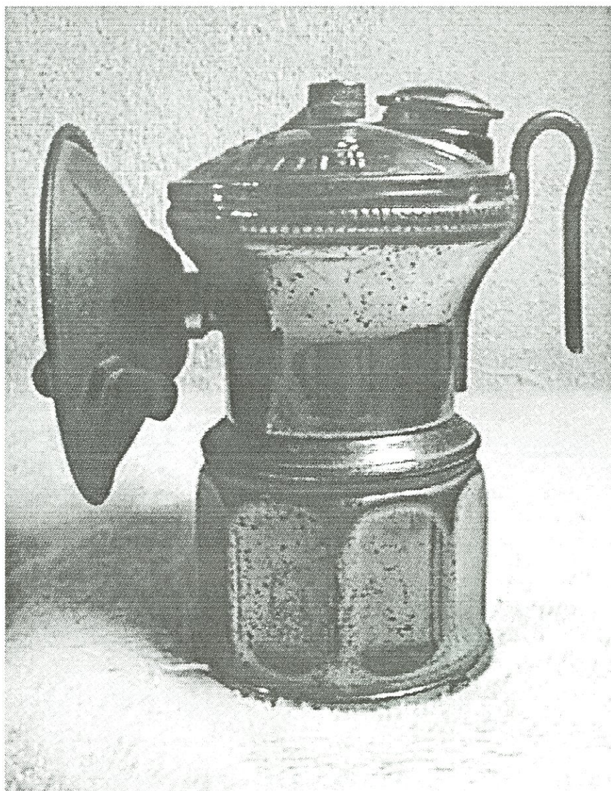
Unfired Elkhorn without cap brace or reflector brace, note long hook.
