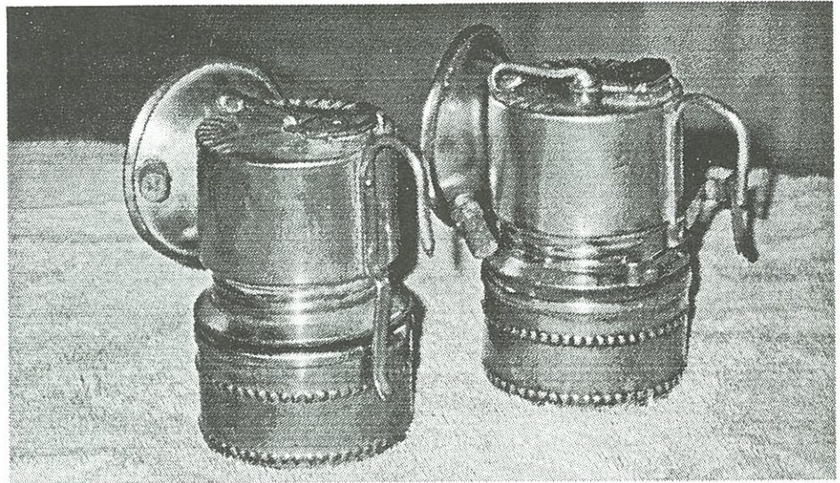
Both lamps are 'Bulldogs': They use a top-mounted water lever.
