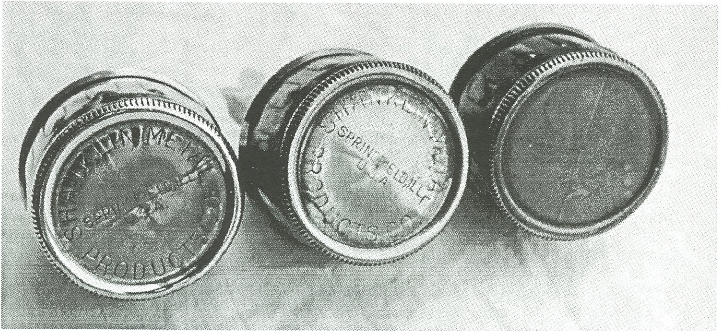
Three base variations: Stamped, stamped and soldered over, and unstamped.
