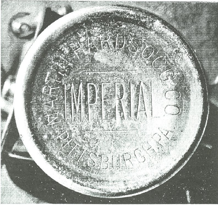
The Hardsocg Imperial cap lamp, nickel-plated. Made by Justrite (Dave Thorpe collection).
