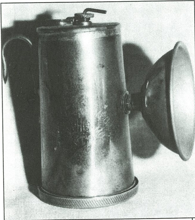
A photograph of the S.E. Simmons carbide lamp. Note the lamp has a reflector similar to a Baldwin deep-dished reflector. (Errol Christman collection)
